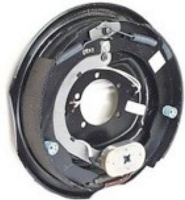
Unlike our cars and trucks, most of our trailers have the old style electric drum brakes that require periodic manually adjustment. Just having good linings isn't enough to stop you -- the brakes must be properly adjusted.
